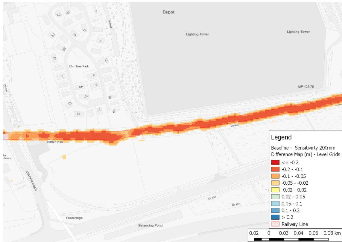
Figure 17: Flood level difference map for comparison between the Baseline run and the 200mm railway level sensitivity run at Station Road (1% AEP in 2115).
